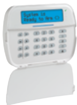
HS2LCD Full Message LCD Keypad
